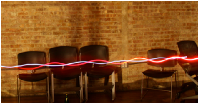
Figure 2: Long exposure photograph indicating out of phase movement of the COMs of the load and the subject. The white light is on the subject, red light is on the bag.
